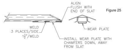
b. Place wear plate support assembly under wear plate, attached to the bottom of the floor slat. Make sure that the two faces of the hardened wear plates are in contact and weld the formed angle mounts to the 45° sloped baffle.
