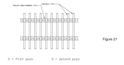
See Figures 22 & 23 for welded and bolted sub-deck details. Mylar tape or paint should separate aluminum profiles from steel cross-members to prevent metal decay.
