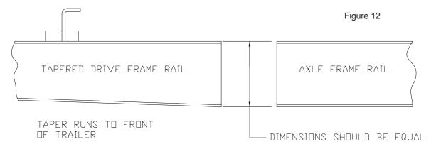
**NOTE:** Exact alignment of trailer centerline with the drive unit centerline is more important than alignment of the drive unit frame with the trailer's axle beams.
