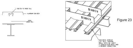
ALUMINUM SUB-DECK ATTACHMENT TO STEEL CROSS SILL
