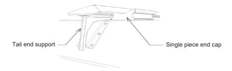
**Note 1:** Tail end supports need to be added after the floor slats are installed to ensure proper installation height.
