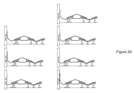
Side seal should span the entire length of the sub-deck. One section of each side may need to be cut, as side seal comes in 12' lengths for steel and 10' lengths for alumimum.
