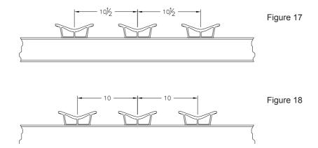
Start at the rear of the trailer. Lay out the sub-deck in the trailer and separate them with spacing jigs, aligning the centerline mark on the jigs with the centerline mark on the cross-member. Keeping the jigs above the cross-members, clamp the jig and sub-deck to every other cross-member. Sub-decking should start 11" inside the rear door and end 6" from the front wall (Figure 19).
